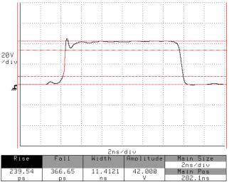
The AVI series provides high amplitude (up to 100) Volts) pulses with rise times as low as 100 ps.
