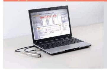
Connect the pyrometer PYROSPOT DT 25L with the optionally available USB parameterization cable (part number: 3310A14012) to a computer. The software PYROSOFT Spot must be installed on thic PC.
