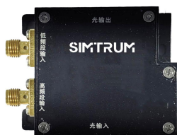
Free Space Acousto-Optic Modulators (AOM)
