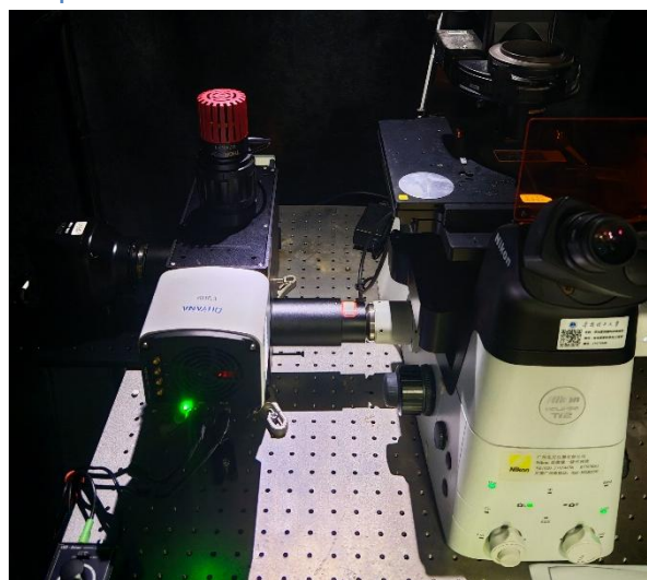
Multi-channel Fluorescence Module 1. Switching optical path 2. Dual-channel optical path switching with replaceable filters 3. Three-channel optical path switching with replaceable filters
