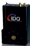
Visible Single-Photon Detector (Peak QE ~ 800nm)
