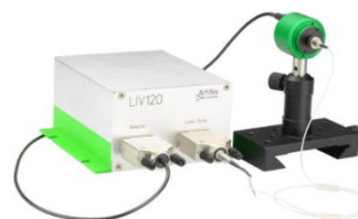
Laser Diode Characterization System LIV120
