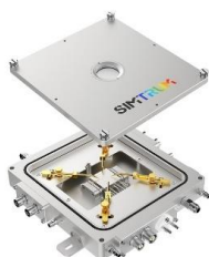
Electrical Probe Temperature Stage -190 ~ 600 °C
