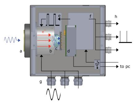
When the TRiCAM is mounted to a microscope or lens, the incoming light (a) is focused onto the entrance window of the image intensifier (b). The image intensifier converts the optical image to electrons, amplifies this electron image, and re-converts the electrons into photons. A fiber-optic taper (c) guides the amplified optical image to the CMOS module for registration and read-out (d).
